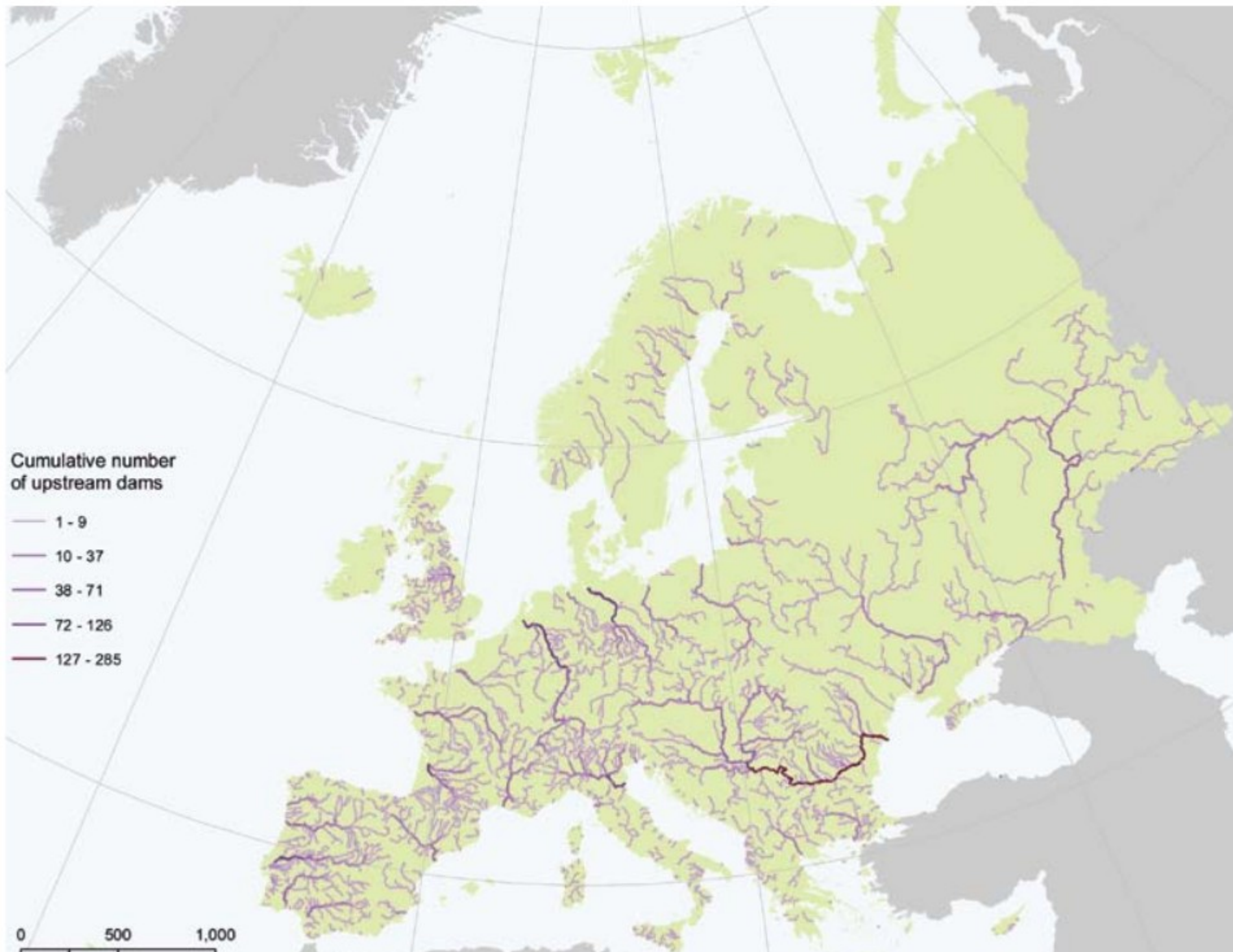
Figure 10. Cumulative number of upstream dams on major European rivers. From Mulligan et al. 2009.
