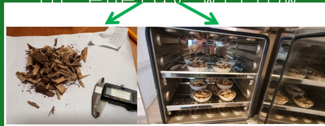
Dimensional characteristics of wood chips and their moisture content for short-rotation crops of energy willow
